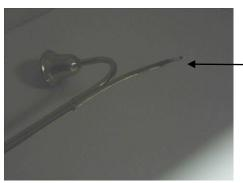
When the end of the holder is push forward and the needle-like eye hole exposed, it is time to "thread" the thin, wax covered wick through the eye hole. (Note: The spare wicks are stored in the third cabinet behind the altar (on the tabernacle side)).
