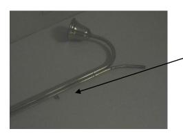
Push the wick holder lever forward (toward the bell) to expose the end of the holder (which has a needle-like eye hole on its end when exposed).
